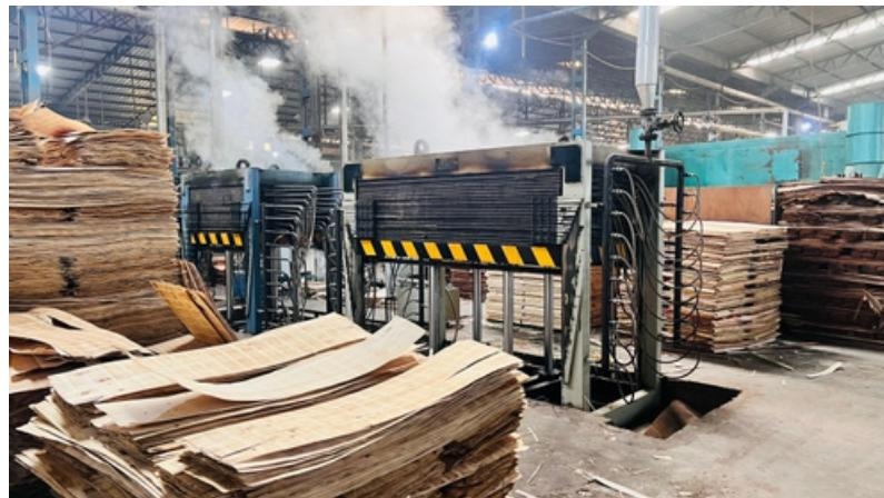
MMC's Has Different Uses And Application In Wood Industry. Fitted With High Powered Cylinders And Hot Platen, These Products Provide High And Delay Free Performance. The Medium In Such Type Of Products Can Be Steam Oil Or Hot Stream Depending On The Needs Of The Client.
