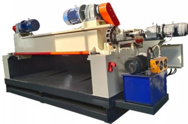
The spindle less wood log debarker machine is used to remove the log bark and make it round before veneer peeling. This machine has hydraulic system. It adjusts the open size by the hydraulic system, that can guarantee the log is firm when the log is removed the bark. The basic model size is 4ft, 8ft. The wood log debarker can be customized according to the wood log diameter , wood log length and the wood log type .
