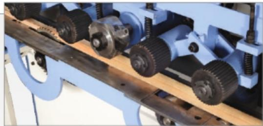
Specially designed machine to convert peeled waste wood round stick in to square bit, which can be used as a filler material in flush door/ block board.
